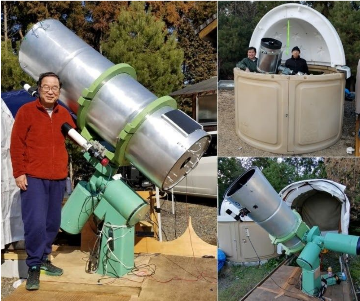
45cm Newtonian telescope (hand made tubu assembly)
